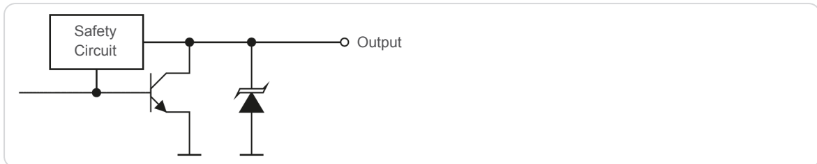
Fig. 14: Principle schematic diagram of the NPN outputs
