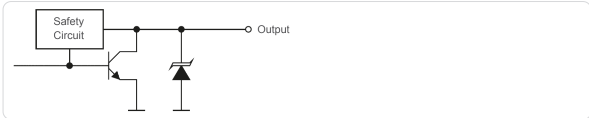
Fig. 14: Principle schematic diagram of the NPN outputs
