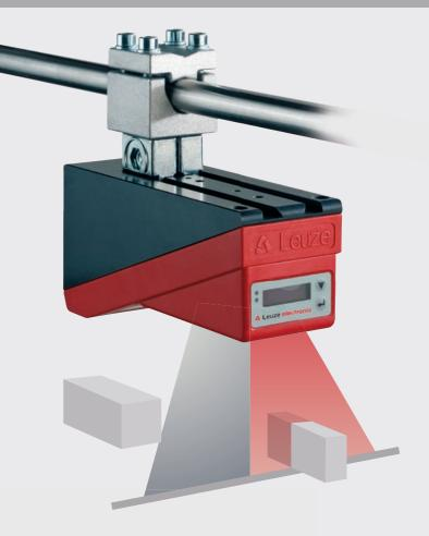
Line Range Sensors are designed to perform proximity object detection along the laser line. Similar to a light barrier or a laser scanner, the sensor detects the presence of objects through scanning. With individual configuration, one sensor can be used to detect single or multiple objects.
