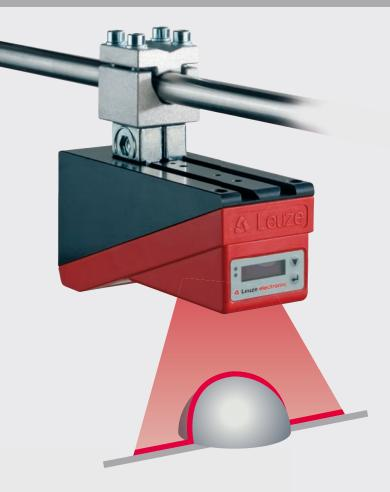
The LPS sensor is used wherever sizes and positions of stationary or moving objects are to be measured. An additional encoder connection permits the creation of 3D data when scanning moving objects. This opens up a large range of application possibilities in position, contour and volume measurement.
